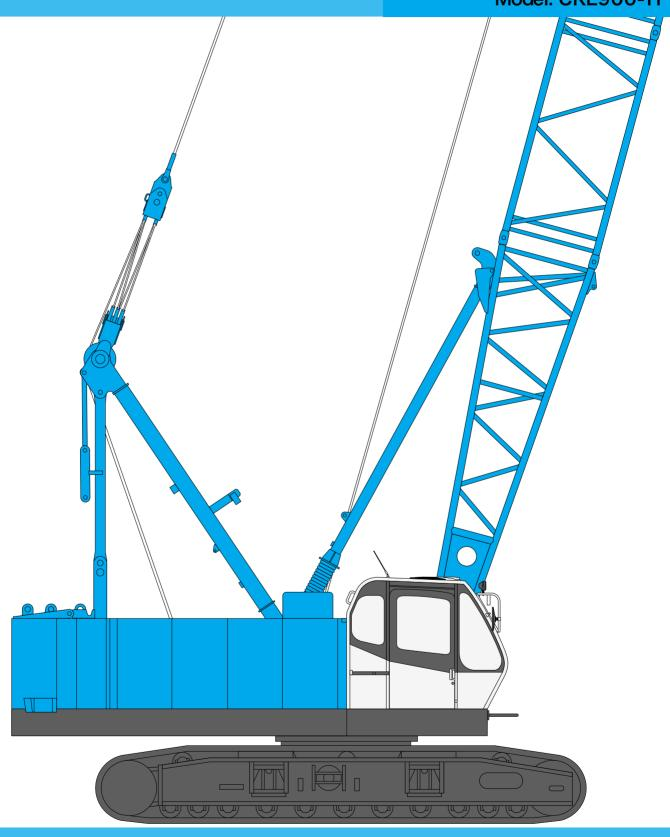
Max. Lifting Capacity: 90 t x 3.4 m Max. Crane Boom Length: 61.0 m Max. Fixed Jib Combination: 51.8 m + 18.3 m
